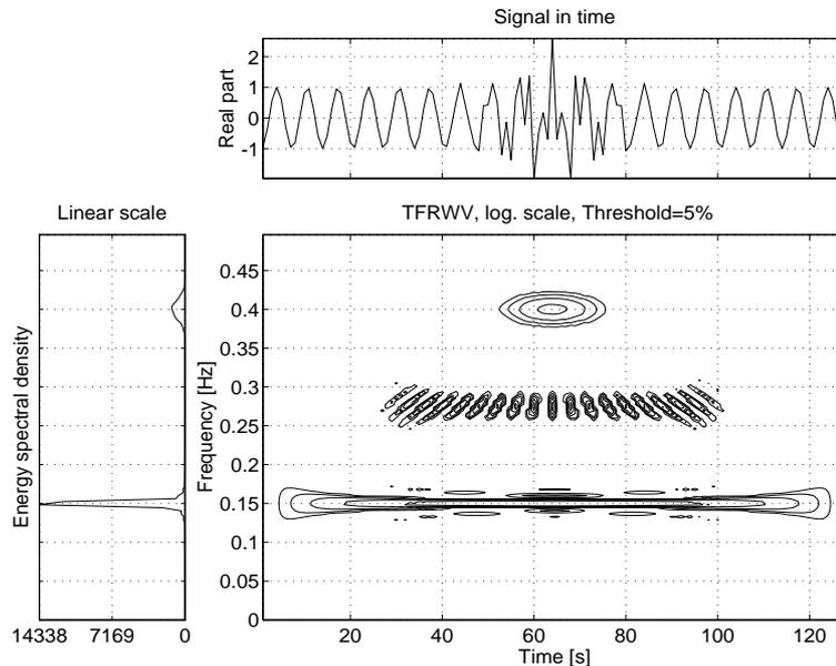
Figure 4.8: WVD of a signal composed of a Gaussian atom and a complex sinusoid. Interferences are present between the two components
