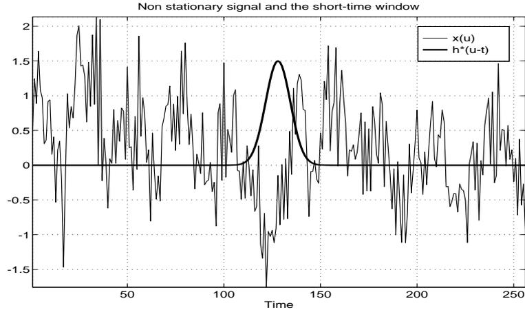
Figure 3.1: non-stationary signal  $x(u)$  and the short-time window  $h^*(u - t)$  centered at time  $t$
