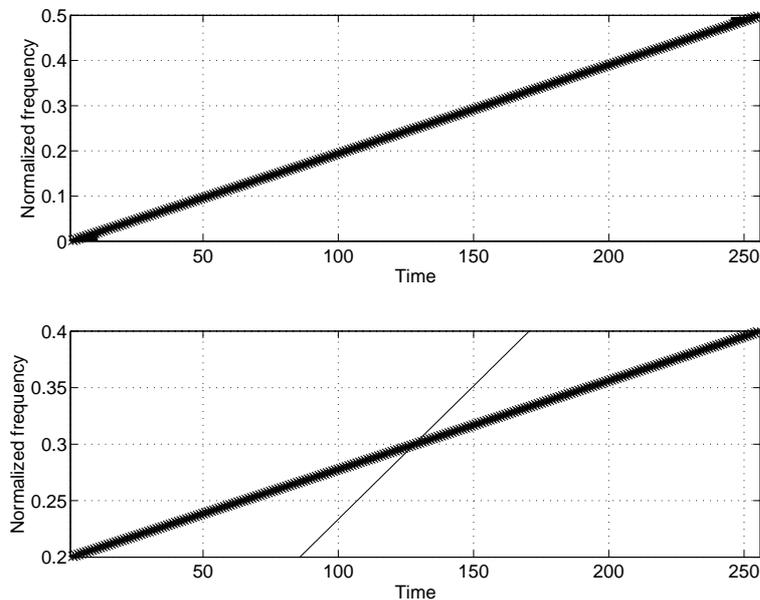
Figure 2.5: Estimation of the instantaneous frequency (stars) and group delay (line) of two different chirps with different amplitude modulations. The first plot corresponds to a large  $T \times B$  product while the second corresponds to a small one
