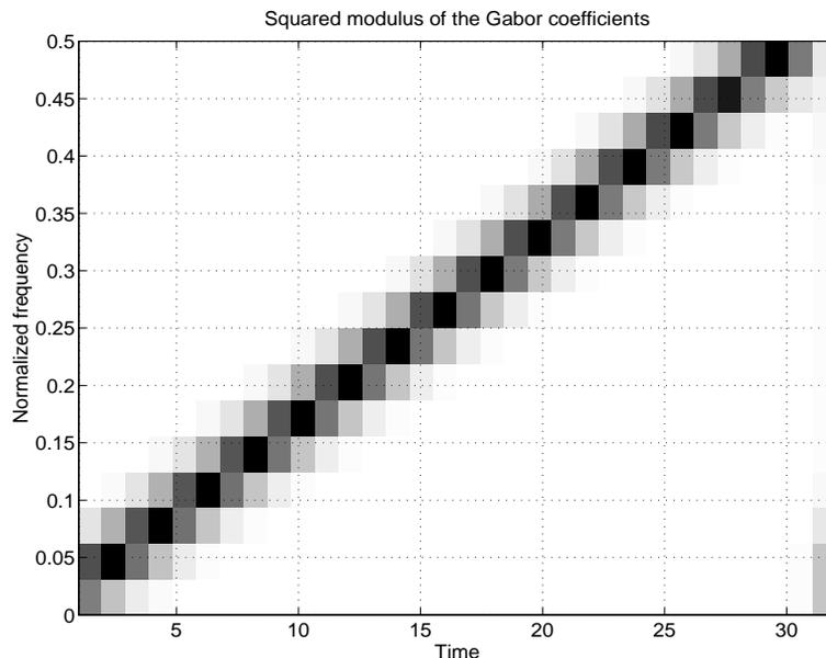
Figure 3.13: Gabor representation of the same chirp, but with a degree of oversampling of 4 : some redundancy improve the readability of the representation
