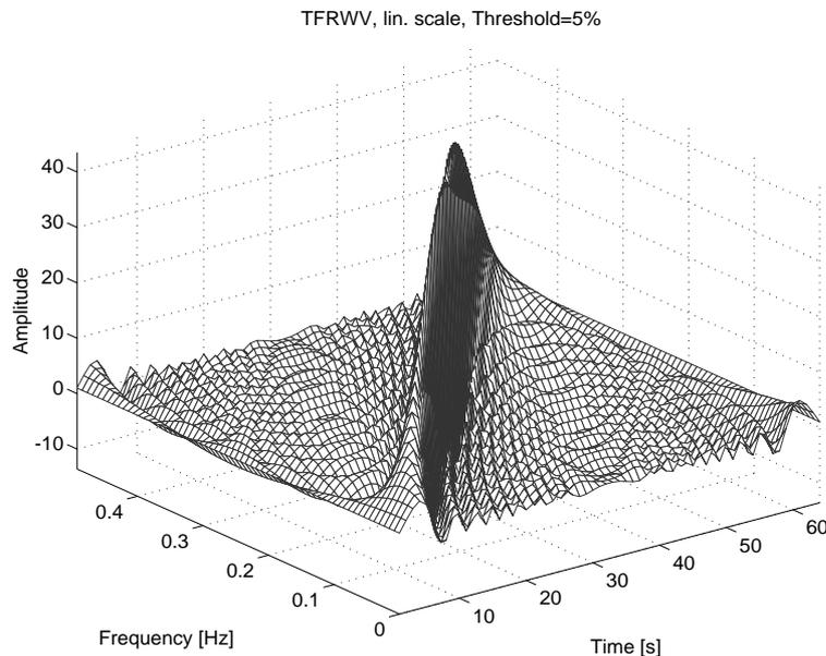
Figure 4.1: Wigner-Ville distribution of a linear chirp signal : almost perfect localization in the time-frequency plane
